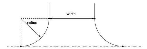
Figure 8.7-1 Driveway Radius and Width Table 8.7-1 Driveway Design Criteria
