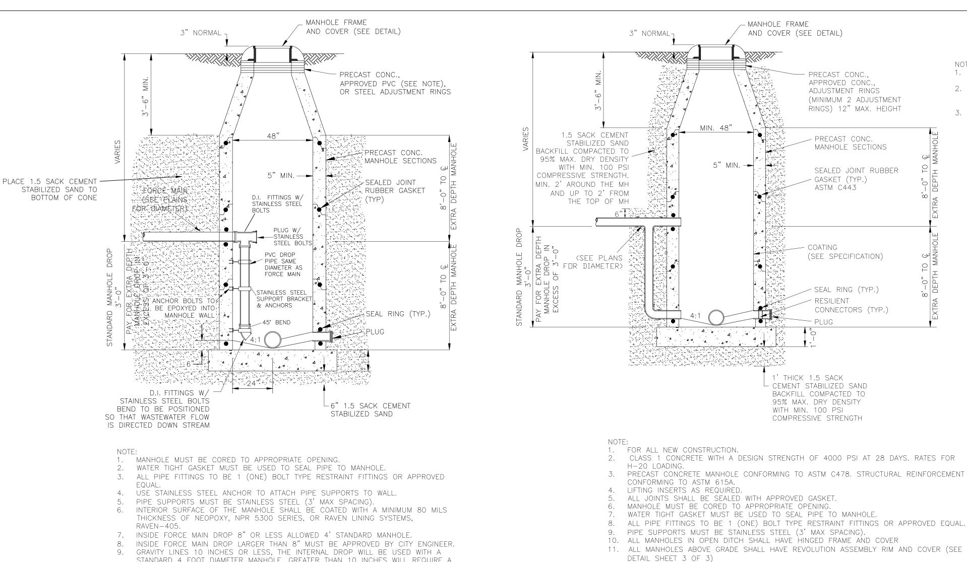
STANDARD 4 FOOT DIAMETER MANHOLE. GREATER THAN 10 INCHES WILL REQUIRE A 6 FOOT DIAMETER MANHOLE.
